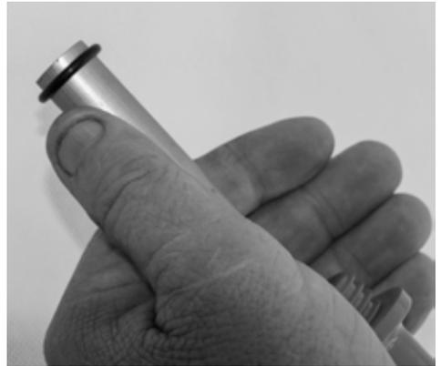
Put 4 drops of thread locker into the female end.
